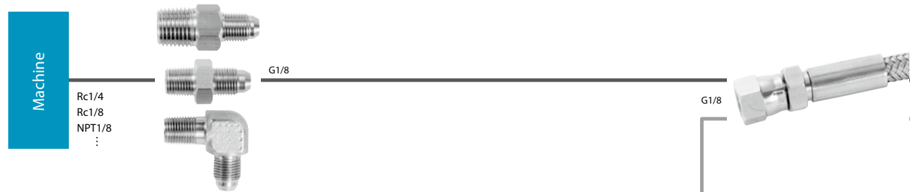
With coupling (Pump pressure: Up to 7.5 MPa)
